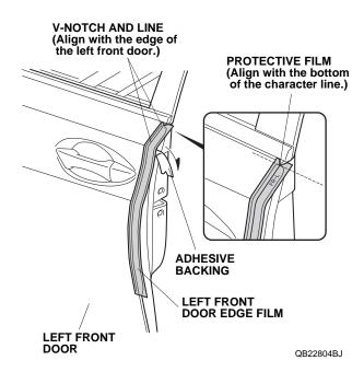
Align the center line on the left front door edge film 8. with the edge of the left front door. While applying light pressure, carefully remove the adhesive backing.
