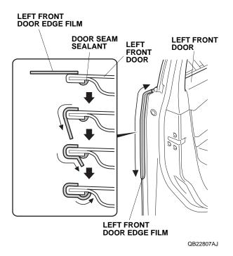
12. Using a shop towel, wipe the excess 3M protective tape application solution from the left front door edge film. Allow the door edge film to dry thoroughly.
