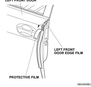
11. Starting from the center and working outward, use your fingers to fold the left front door edge film around the edge of the door as shown. Move your fingers in one direction only. Attach the door edge film over the seam sealant. Do not damage the door seam sealant.
