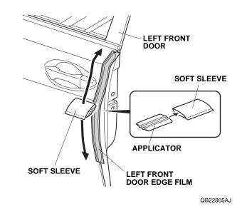
10. Slowly remove the protective film from the left front door edge film.
