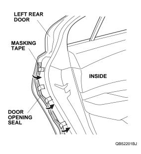
4. Using the alcohol swab, thoroughly clean the area where the left rear door edge film will attach.
